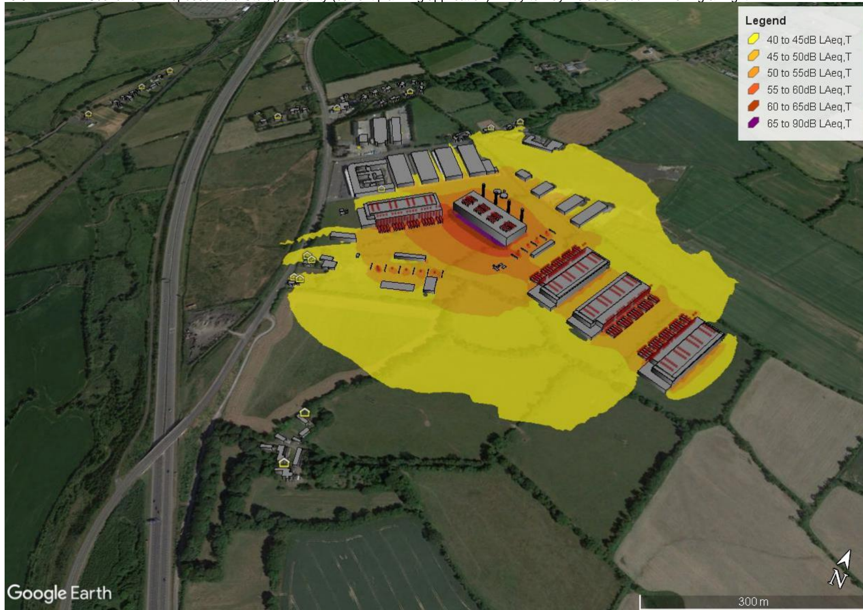
Figure 10.6 Scenario A Proposed Data Storage Facility (current planning application) – Day to Day Noise Contour – Evening & Night
