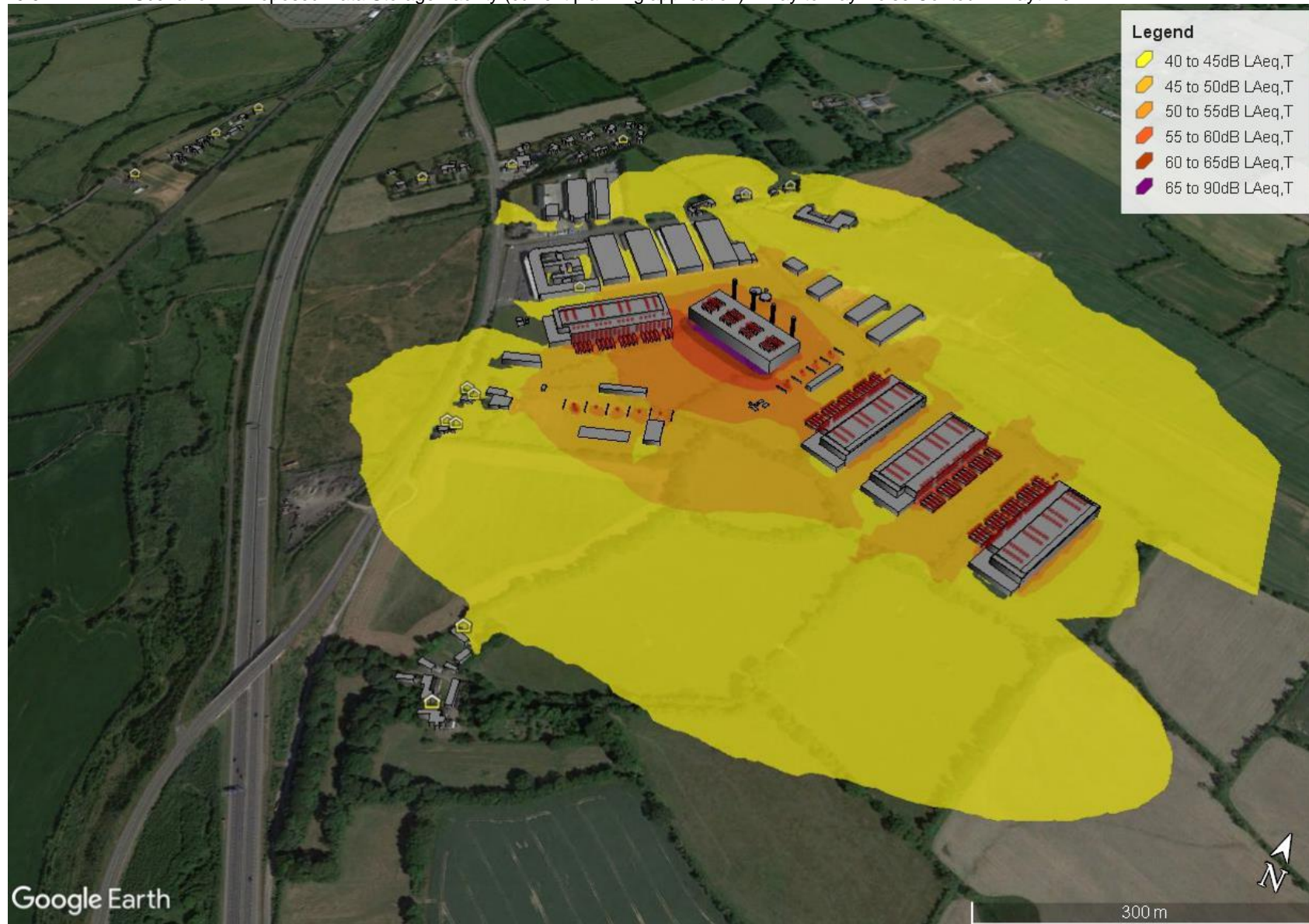
Figure 10.5 Scenario A Proposed Data Storage Facility (current planning application) – Day to Day Noise Contour – Daytime
